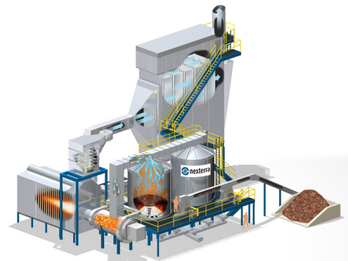
Figure 3: Configuration of 12 MWt Direct Fired Boiler System
